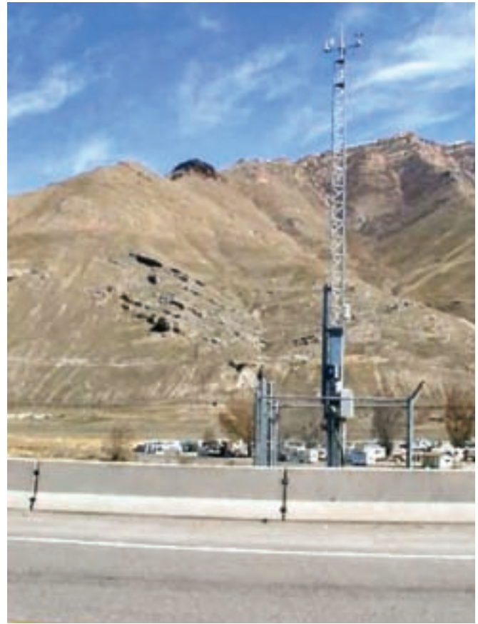
Environmental Sensor Systems with road sensors are the basis of a Road Weather Information System, shown here in Utah (above) and Iowa (below).
