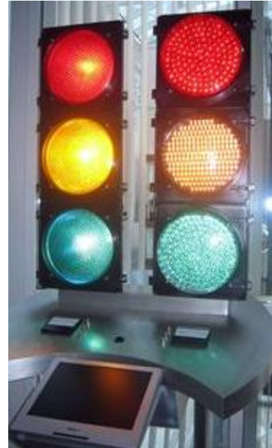
Figure 8. Comparison between incandescent bulb signals (left) and LED signals (right)
