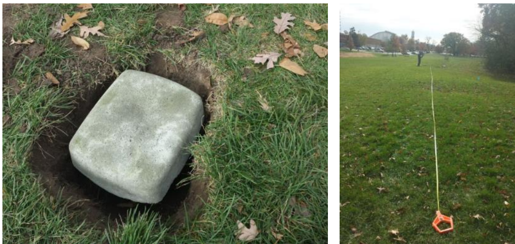
Figure 71. Success rate test: wireless MEMS system inside concrete buried underground (left) and horizontal distance measurement for data transmission (right)
