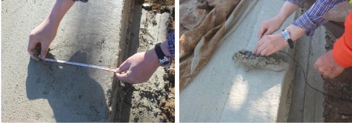
Figure 28. Embedment of MEMS digital humidity sensors
