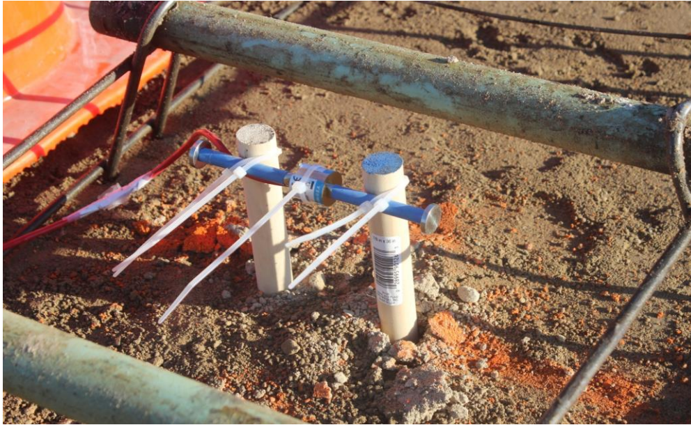
Figure 20. Installation of strain gage at joint
