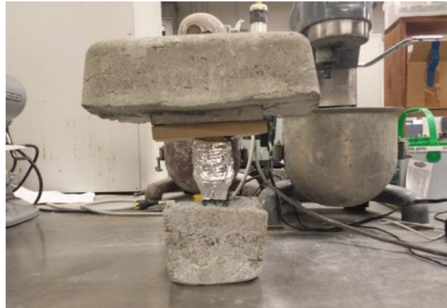
Figure 70. Wireless MEMS system inside concrete
