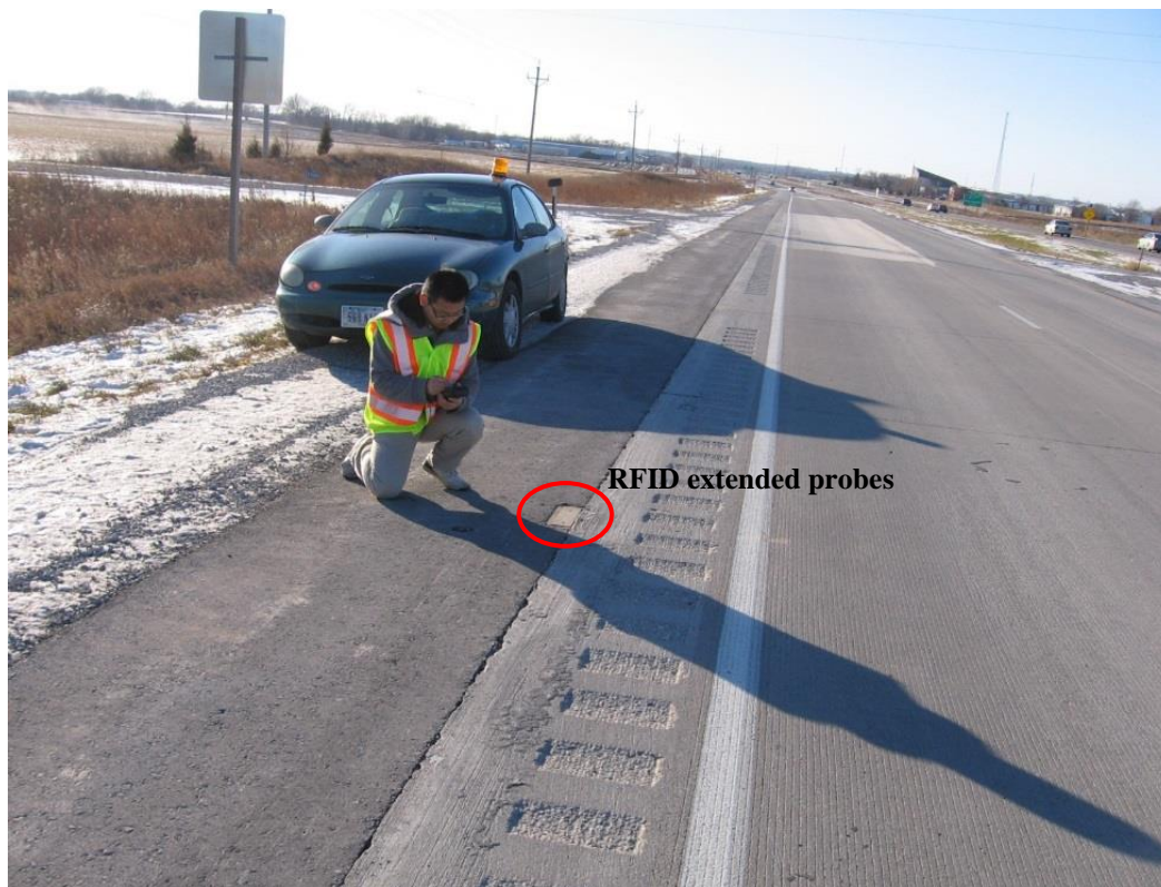
Figure 62. Data acquisition from RFID extended probes in winter
