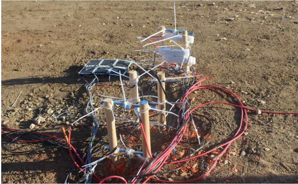
Figure 21. Installation of sensors near the mid-span edge
