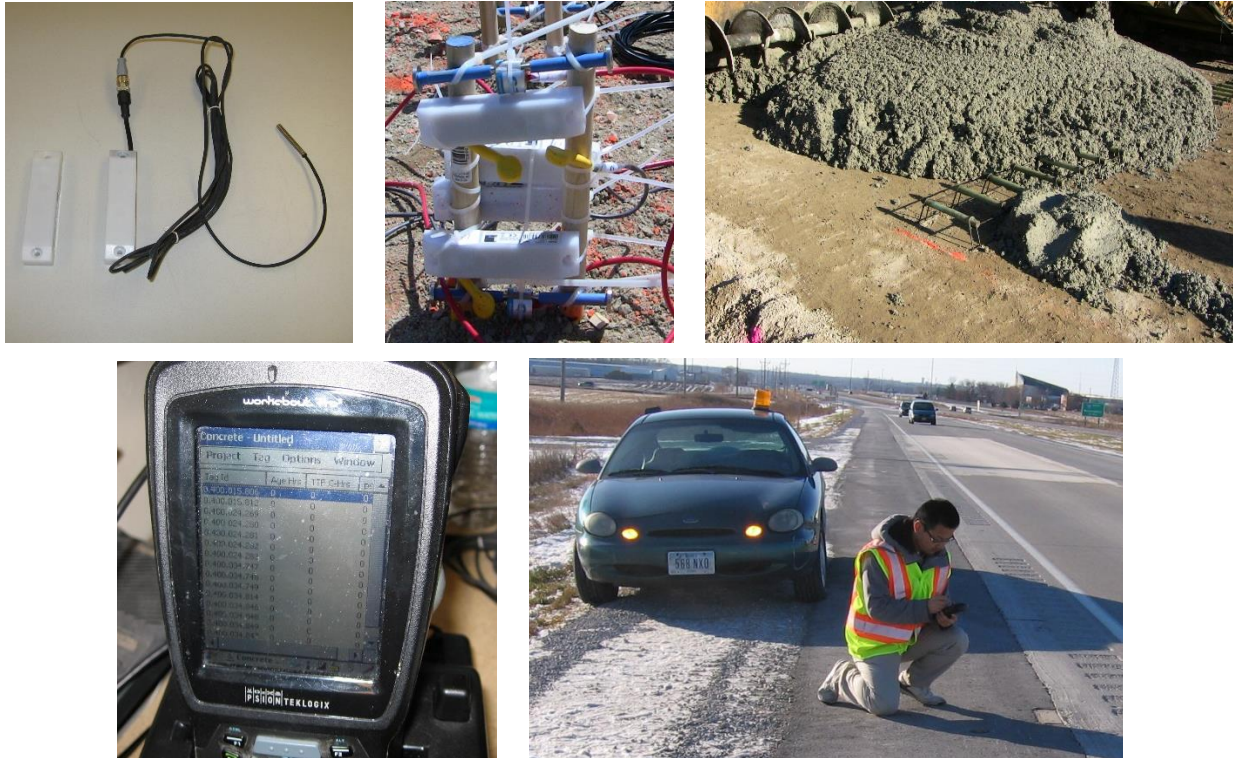
Figure 7. RFID-based wireless concrete monitoring system: RFID tags with/without a temperature probe (top left), installation of wireless RFID tag in the base course (top middle), installation of wireless RFID tag buried in concrete (top right), HardTrack portable with detected wireless RFID tags on the screen (bottom left), data acquisition in the field (bottom right)
