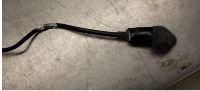
Figure 67. MEMS sensor with packaging
