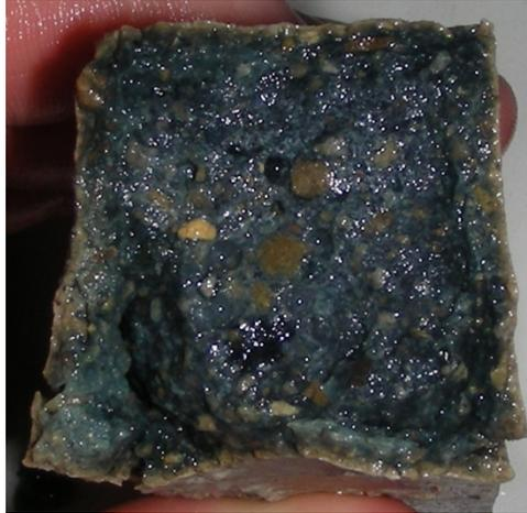
**Figure 3. Internal sulfate attack damage**
