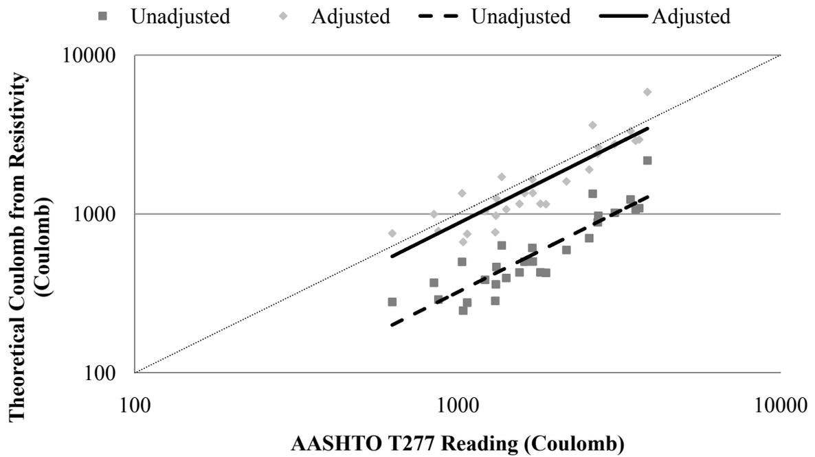
**Figure 36. Geometric correction – T277 coulomb vs. resistivity coulomb**
