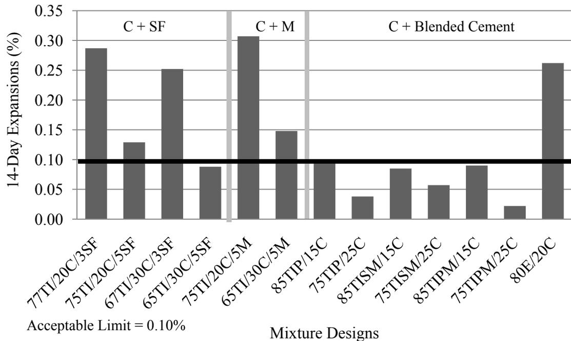
**Figure 7. ASTM C1567 ASR expansion for mixtures containing Class C fly ash blended with silica fume, metakaolin, or blended cement**
