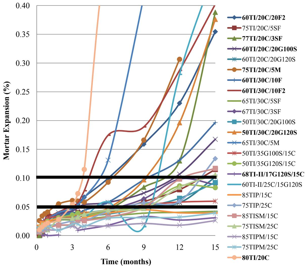
Figure 54. ASTM C1012 sulfate mortar expansions of mixtures containing Class C fly ash
