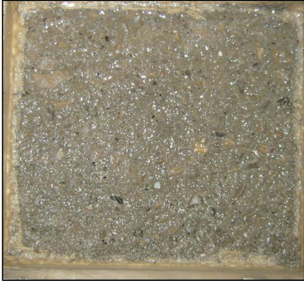
**Figure 45. Visual rating of 3 (moderate scaling, some coarse aggregate visible)**
