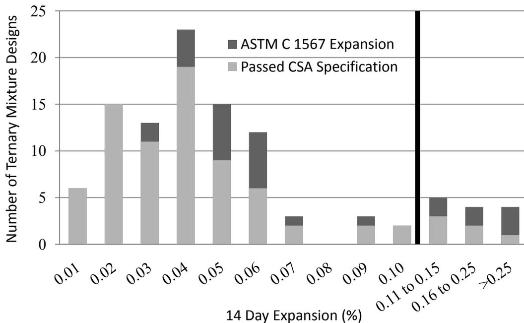
**Figure 25. Number of mixtures for a given expansion that passed CSA standard specification requirements**
