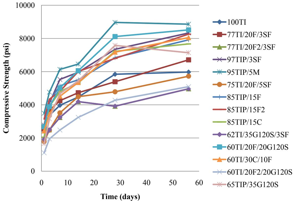
Figure 49. ASTM C39 compressive strength for cold cured mixtures
