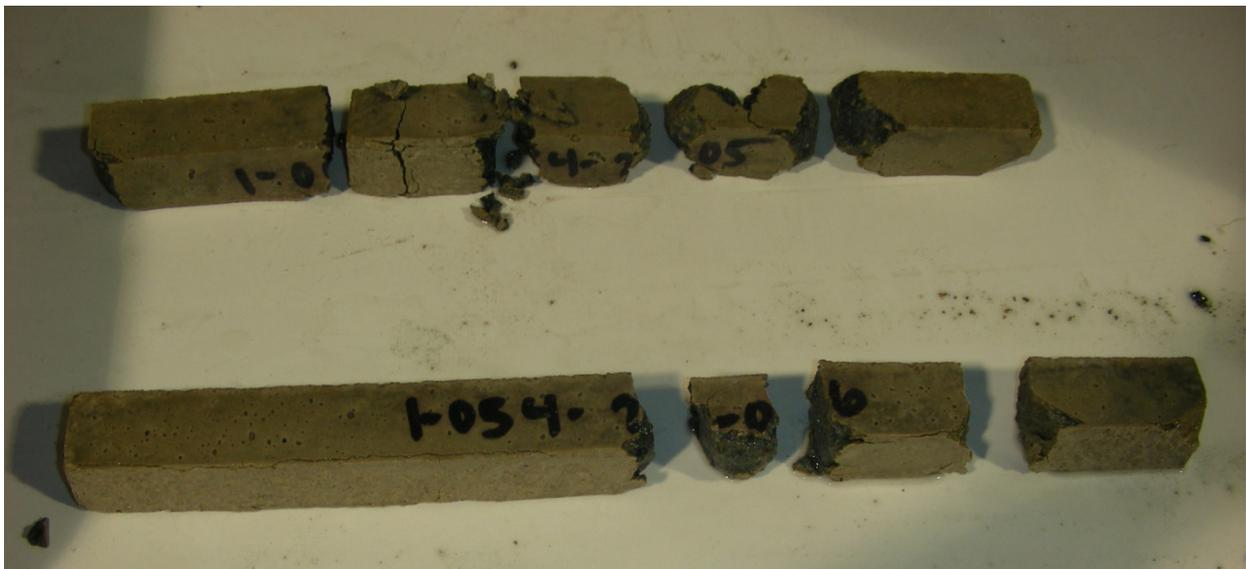
**Figure 4. Severe sulfate damage**
