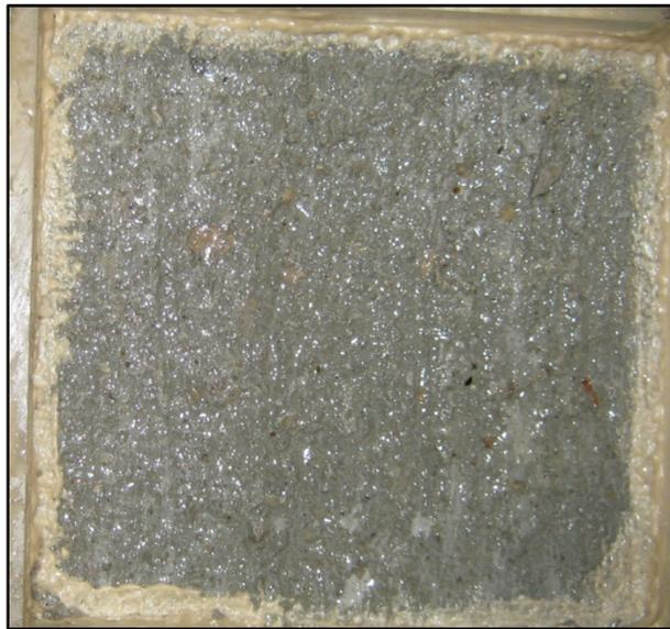
**Figure 44. Visual rating of 2 (slight to moderate scaling)**
