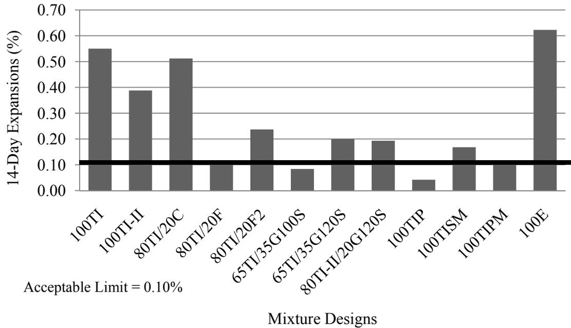
**Figure 5. ASTM C1567 ASR expansion for control mixtures**
