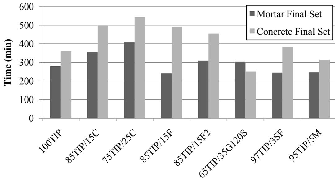
**Figure 28. Final set for Type IP cement mixtures**
