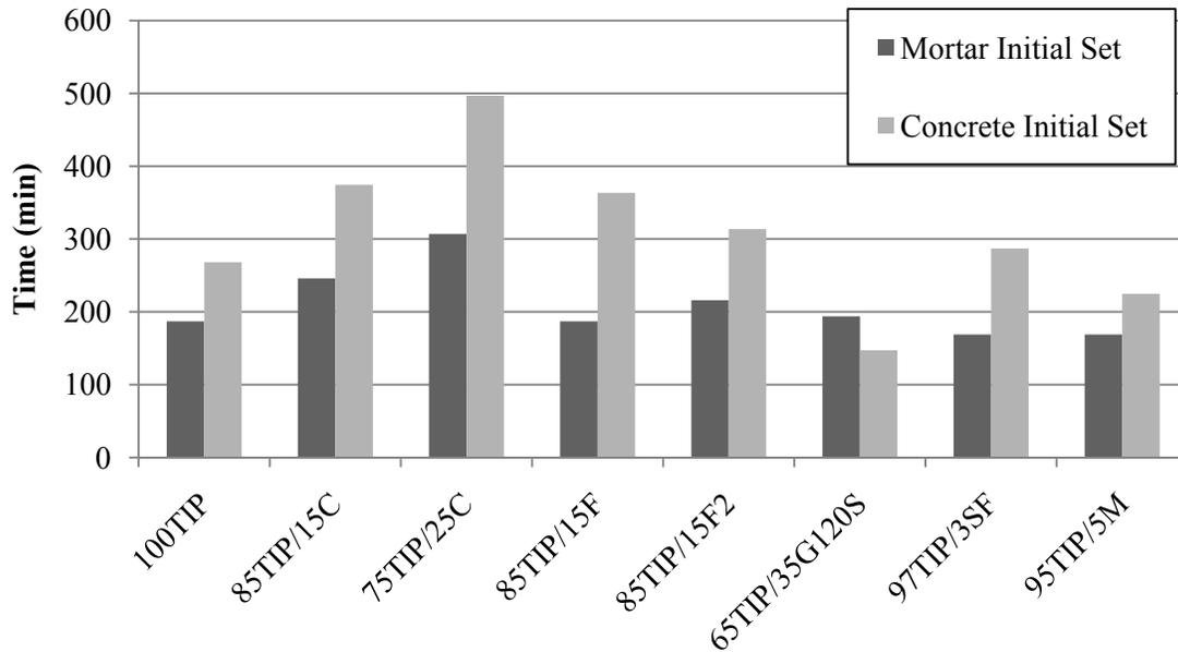
**Figure 27. Initial set for Type IP cement mixtures**
