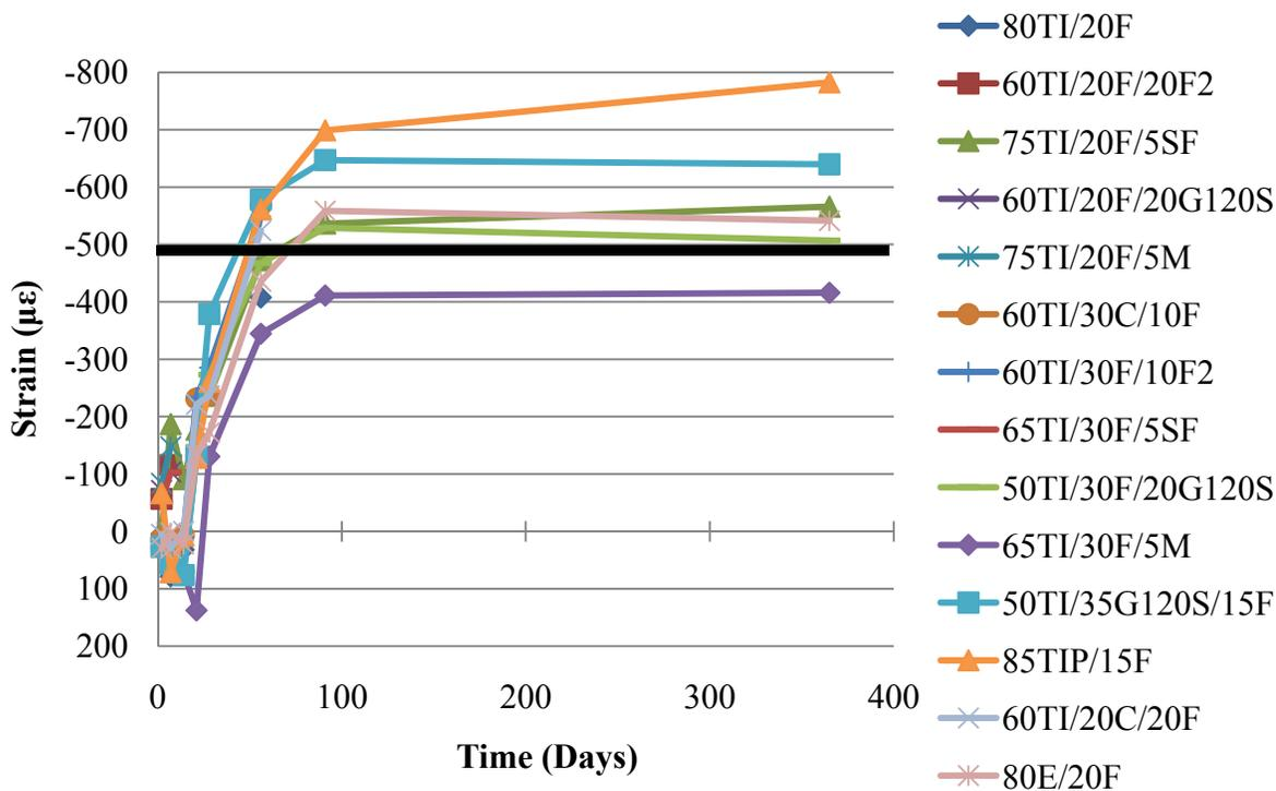
Figure 89. ASTM C157 curing shrinkage strain of mixtures containing Class F fly ash
