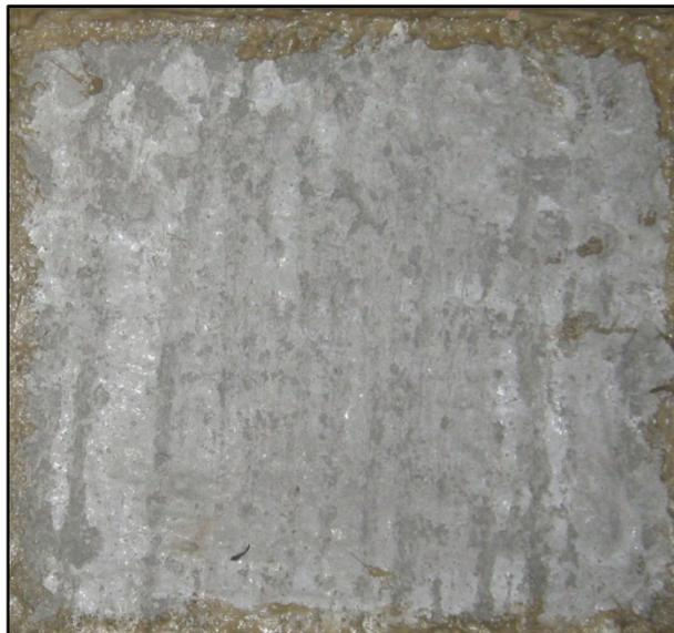
**Figure 42. Visual rating of 0 (no scaling)**
