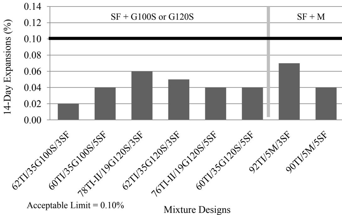
Figure 18. ASTM C1567 ASR expansion for mixtures containing silica fume blended with Grade 100 or 120 GGBFS or metakaolin
