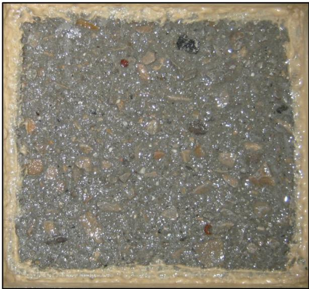
**Figure 46. Visual rating of 4 (moderate to severe scaling)**
