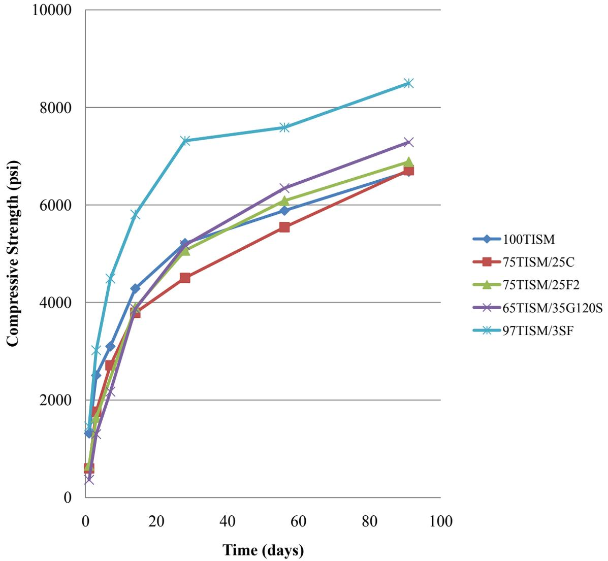
Figure 85. ASTM C39 concrete compressive strengths of mixtures containing Type IS(20) cement
