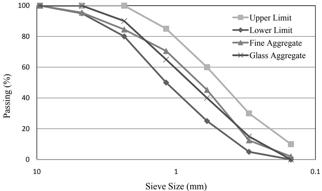
**Figure 1. Gradation of fine aggregates**
