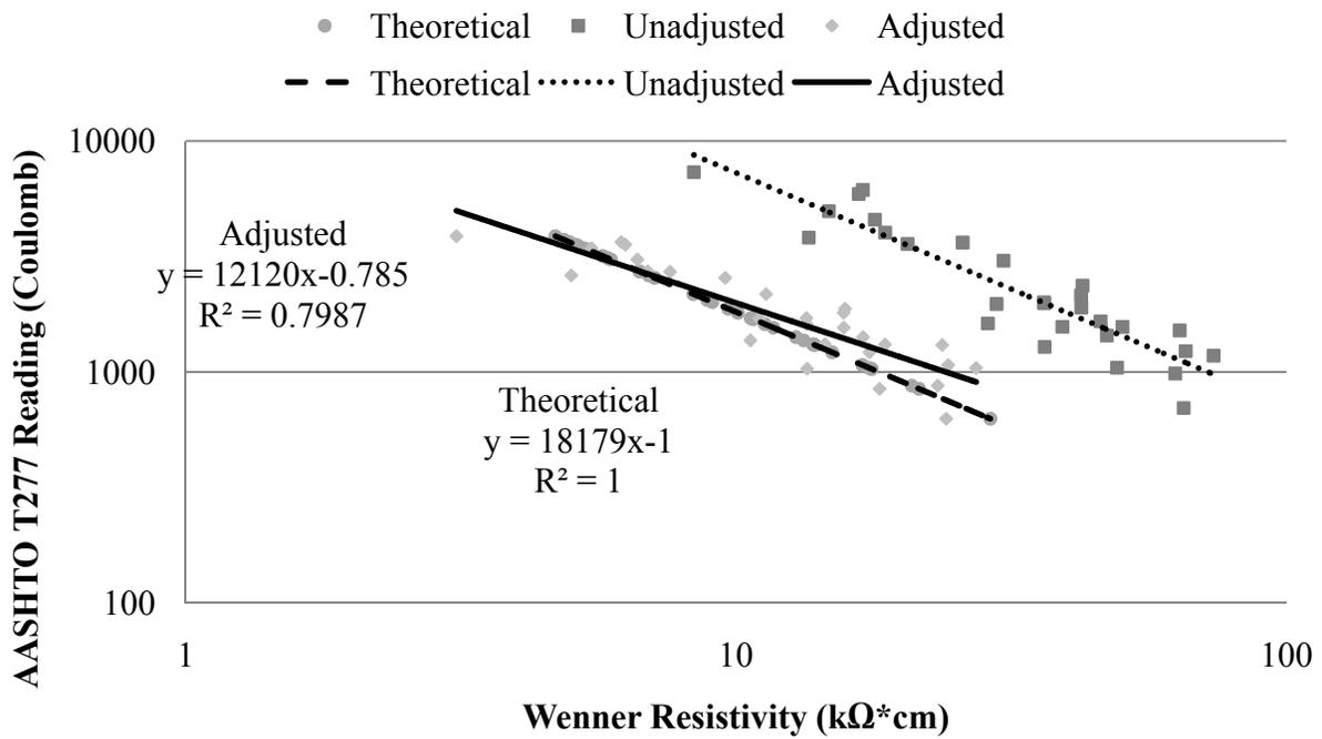
Figure 40. Resistivity vs. AASHTO T277 coulomb (1 in.=2.54 cm)
