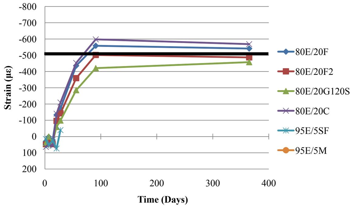
**Figure 96. ASTM C157 curing shrinkage strain of mixtures containing limestone blended cement**
