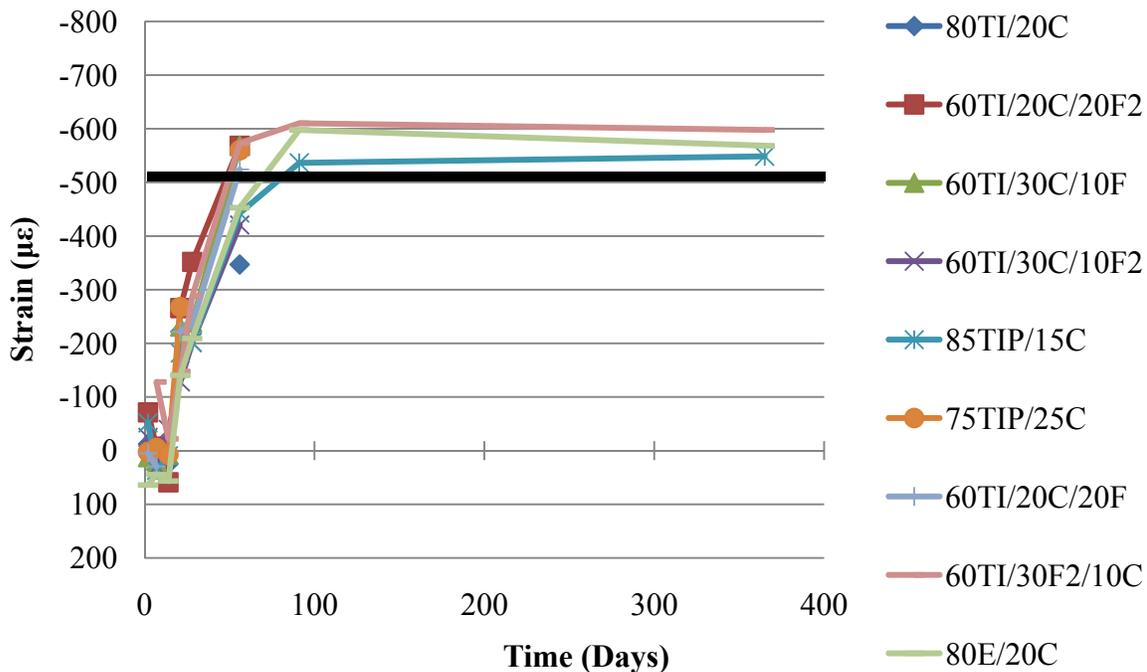
Figure 88. ASTM C157 curing shrinkage strain of mixtures containing Class C fly ash
