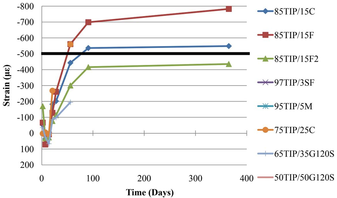
Figure 94. ASTM C157 curing shrinkage strain of mixtures containing Type IP cement
