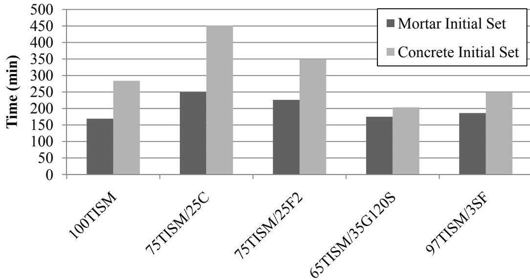
**Figure 29. Initial set for Type ISM cement mixtures**
