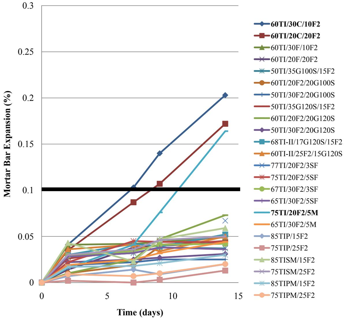
Figure 68. ASTM C1567 ASR mortar expansions of mixtures containing Class F2 fly ash
