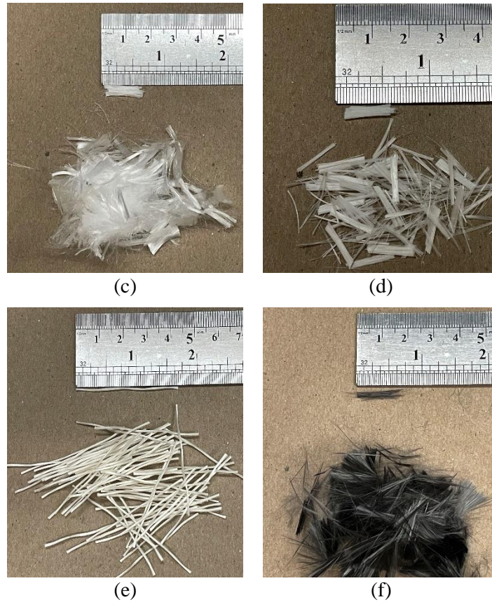
Figure 22. (a) Steel, (b) nylon, (c) PP, (d) PVA, (e) AR glass, and (f) carbon fibers
