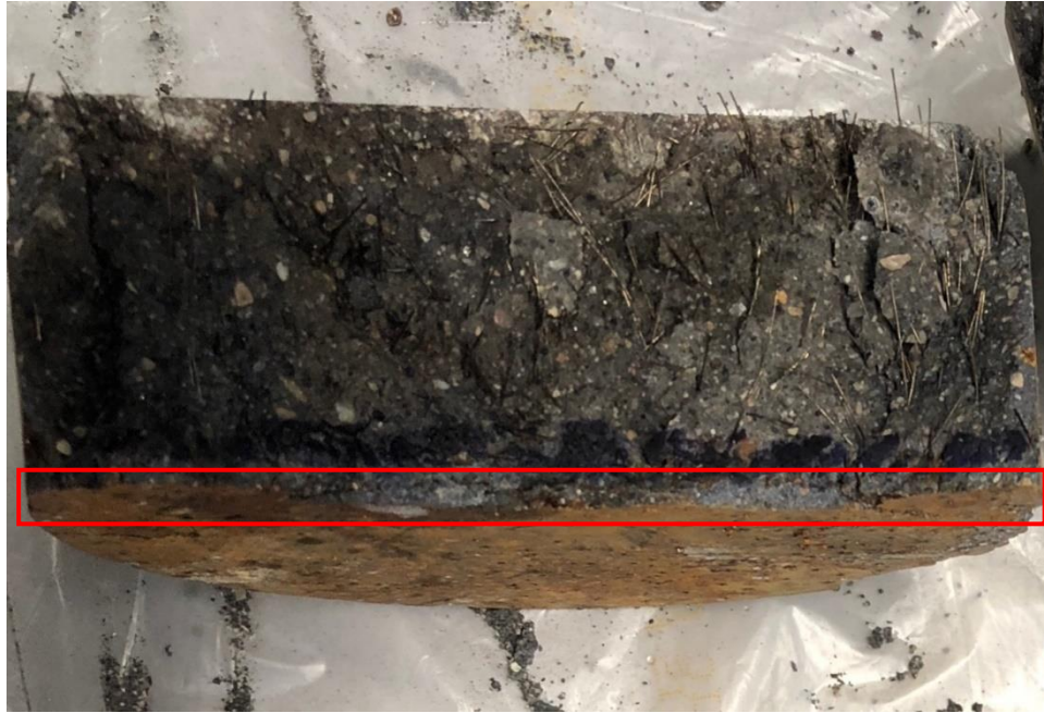
Figure 6. Chloride migration observed in a sample of the NP1 mixture under rapid chloride migration test
