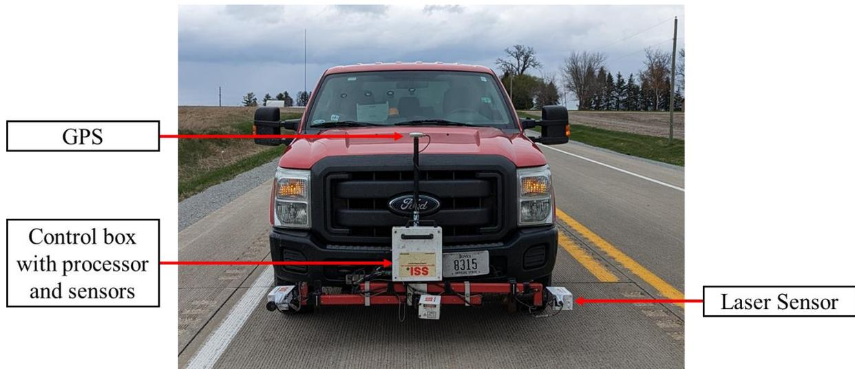
**Figure 4. SSI high-speed profiler**
