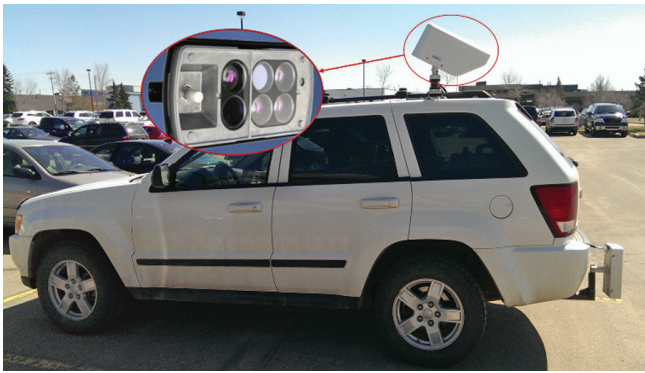
Mobile RWIS unit equipped with spectral road surface temperature sensor
